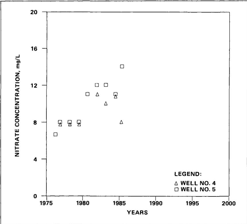
Figure 3. Nitrate concentration trend at Milford, Nebraska (based on data from [18]).
