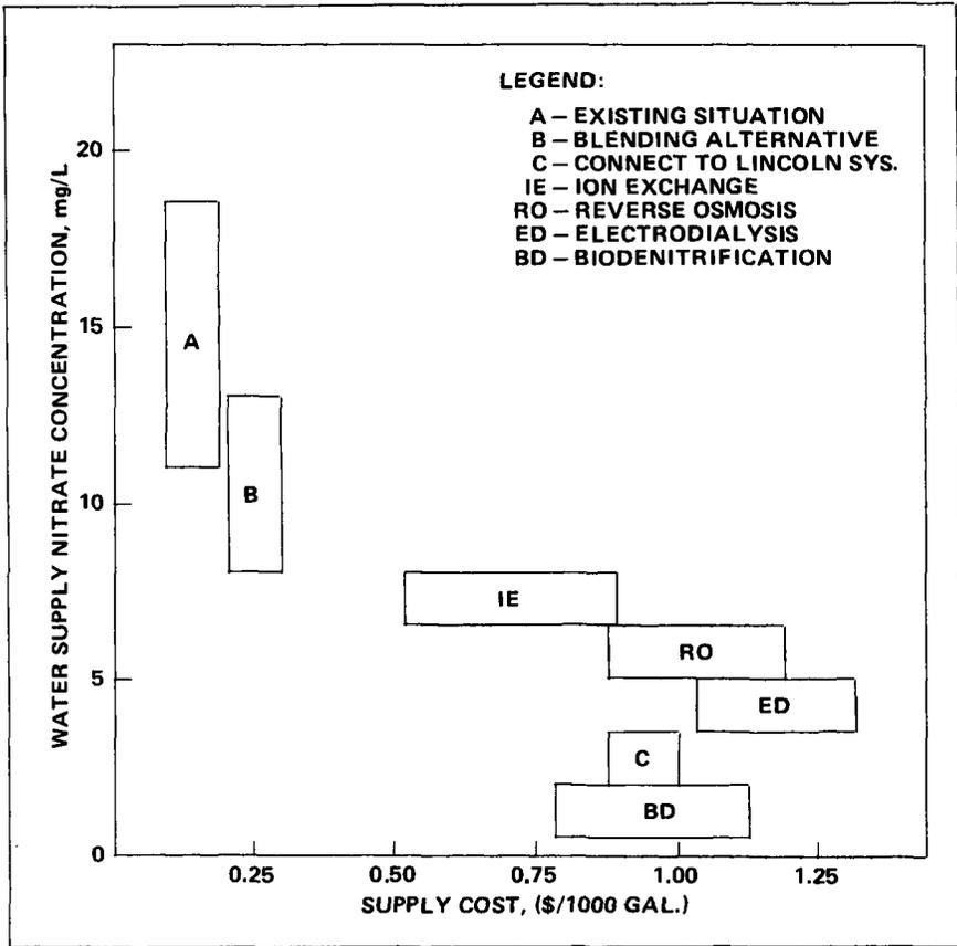
Figure 4. Trade-off between cost and nitrate levels in the water supply for control alternatives available to Milford, Nebraska.
