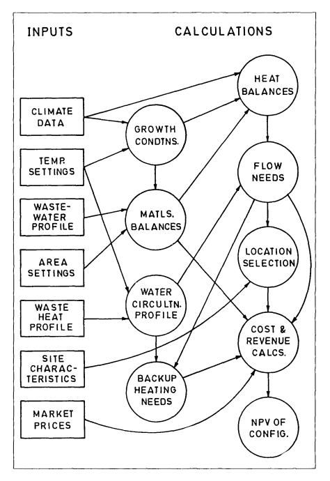
Figure 2. Overview of waste heat utilization assessment methodology.
