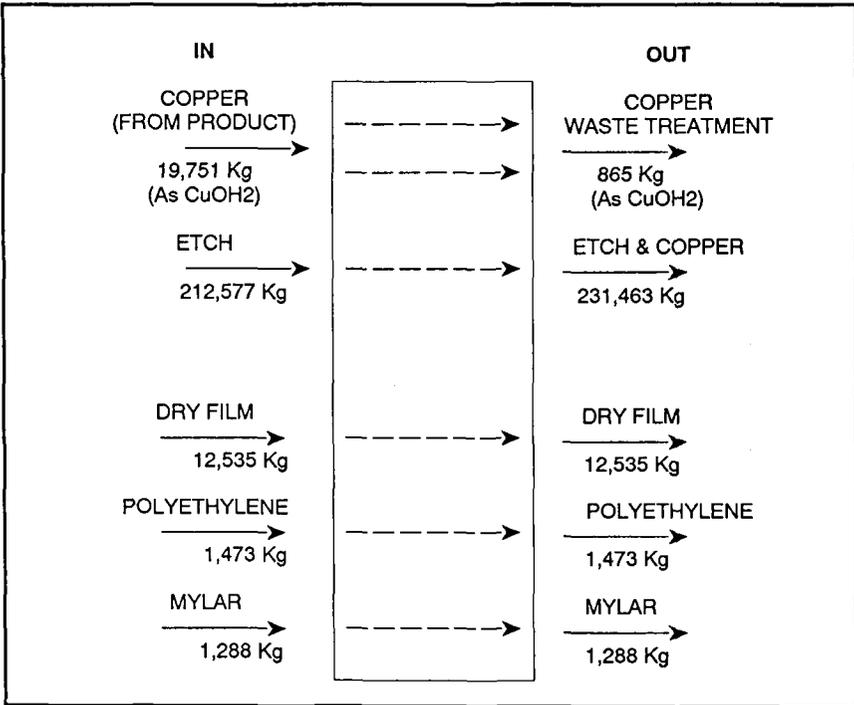
Figure 3. Waste material balance—innerlayer area.
