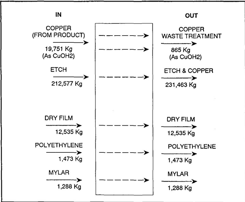
Figure 3. Waste material balance—innerlayer area.
