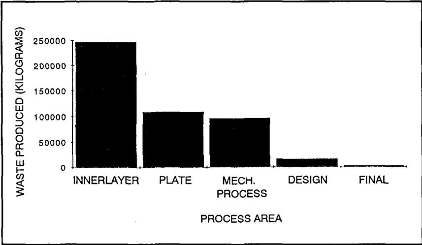
Figure 2. Waste produced in the printed circuit facility.
