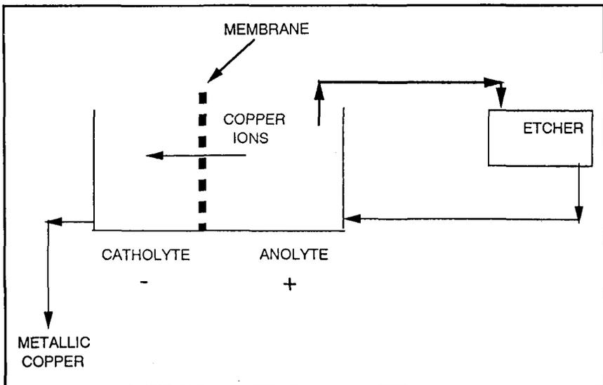
Figure 4. Cupric chloride regeneration system.
