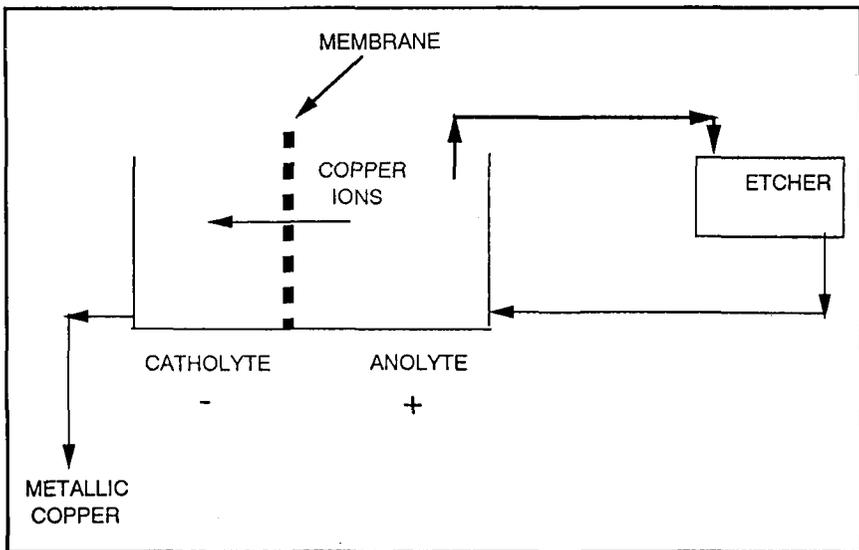
Figure 4. Cupric chloride regeneration system.
