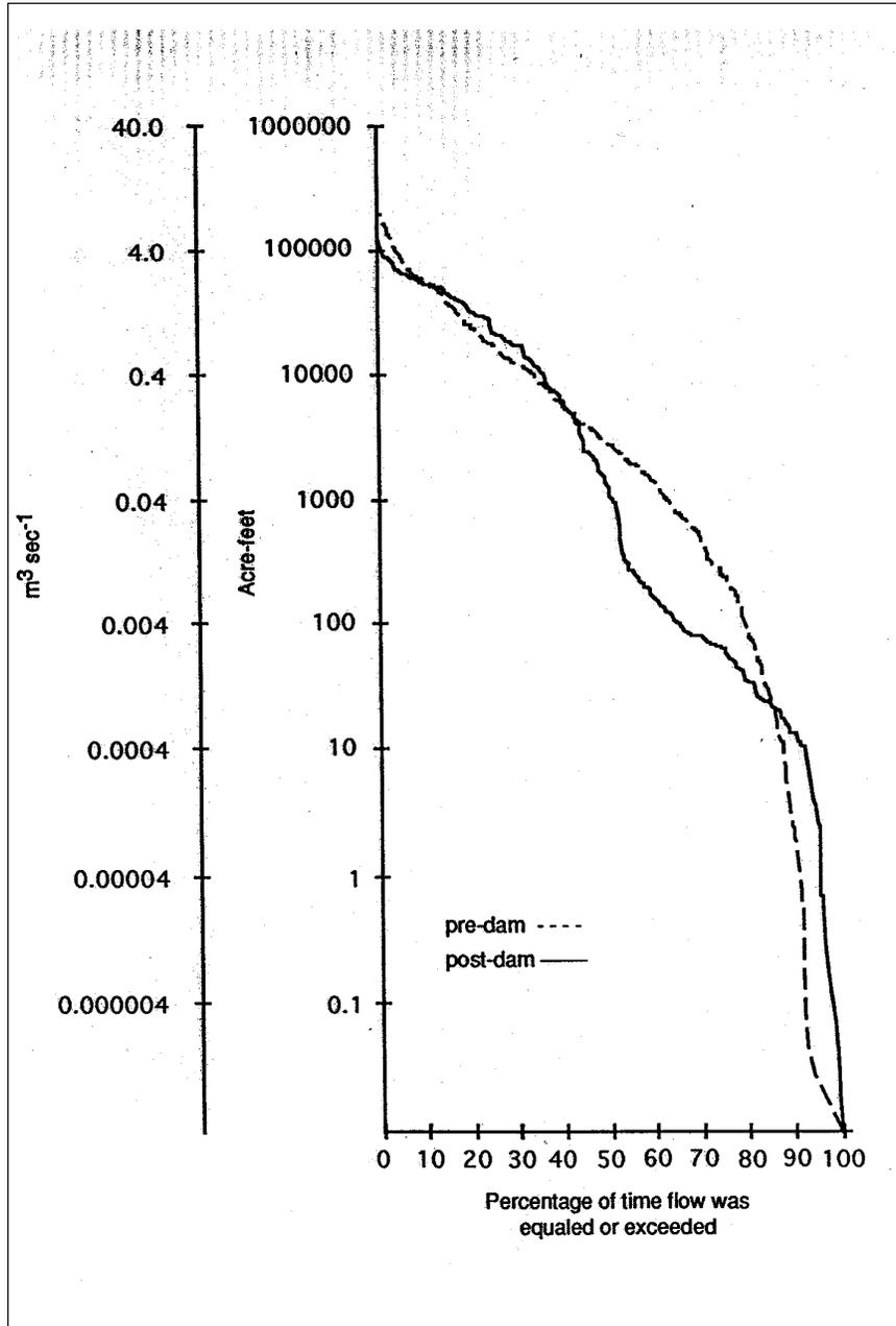
Figure 5. Flow duration curve for Yegua Creek comparing pre-dam and post-dam discharge.
