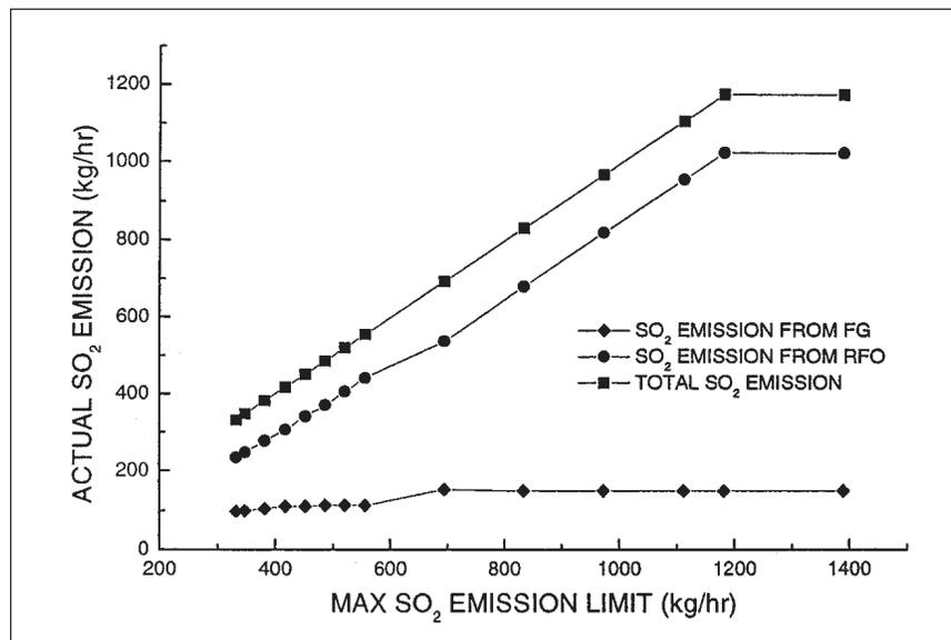
Figure 5. Contributions of  $SO_2$  emissions from fuel gas and refinery fuel oil with free crude mix.
