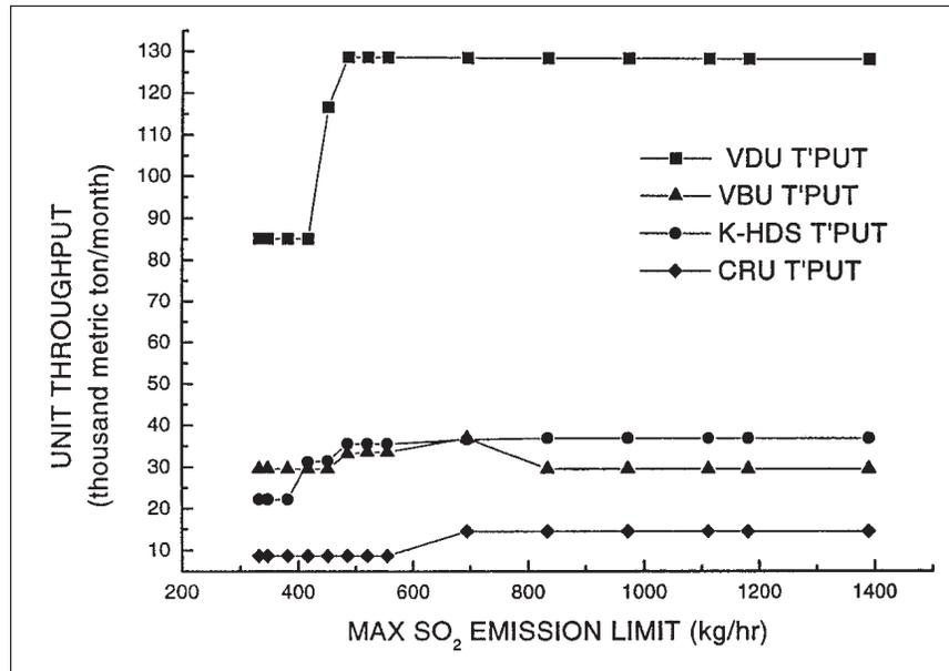
Figure 4. Variations of throughputs of secondary processing units with maximum SO<sub>2</sub> emission limit with free crude mix.
