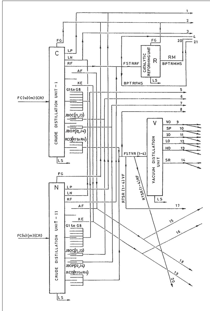
Figure 1. Schematic diagram of various units and streams of the refinery under study (cont'd.).
