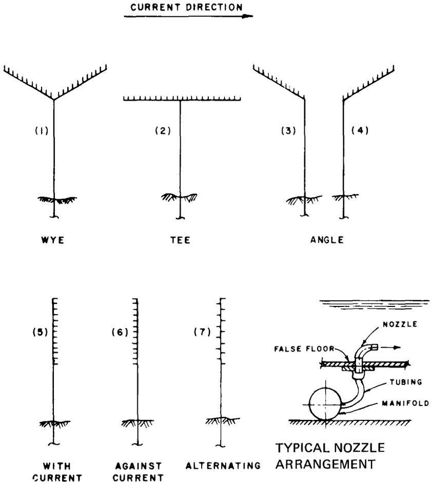
Figure 6. Schematic arrangement of diffuser for phase II model tests.
