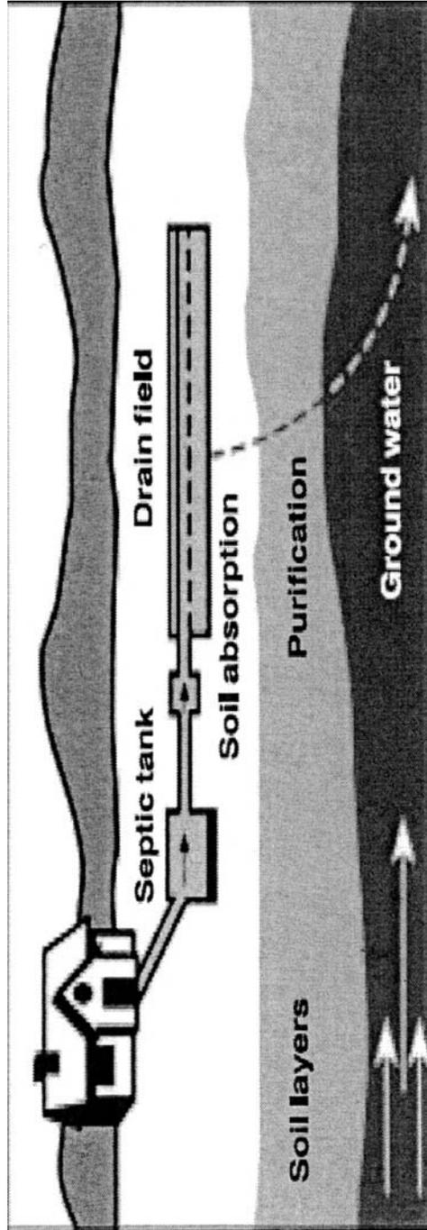
Figure 1. Conventional on-site wastewater treatment system.
