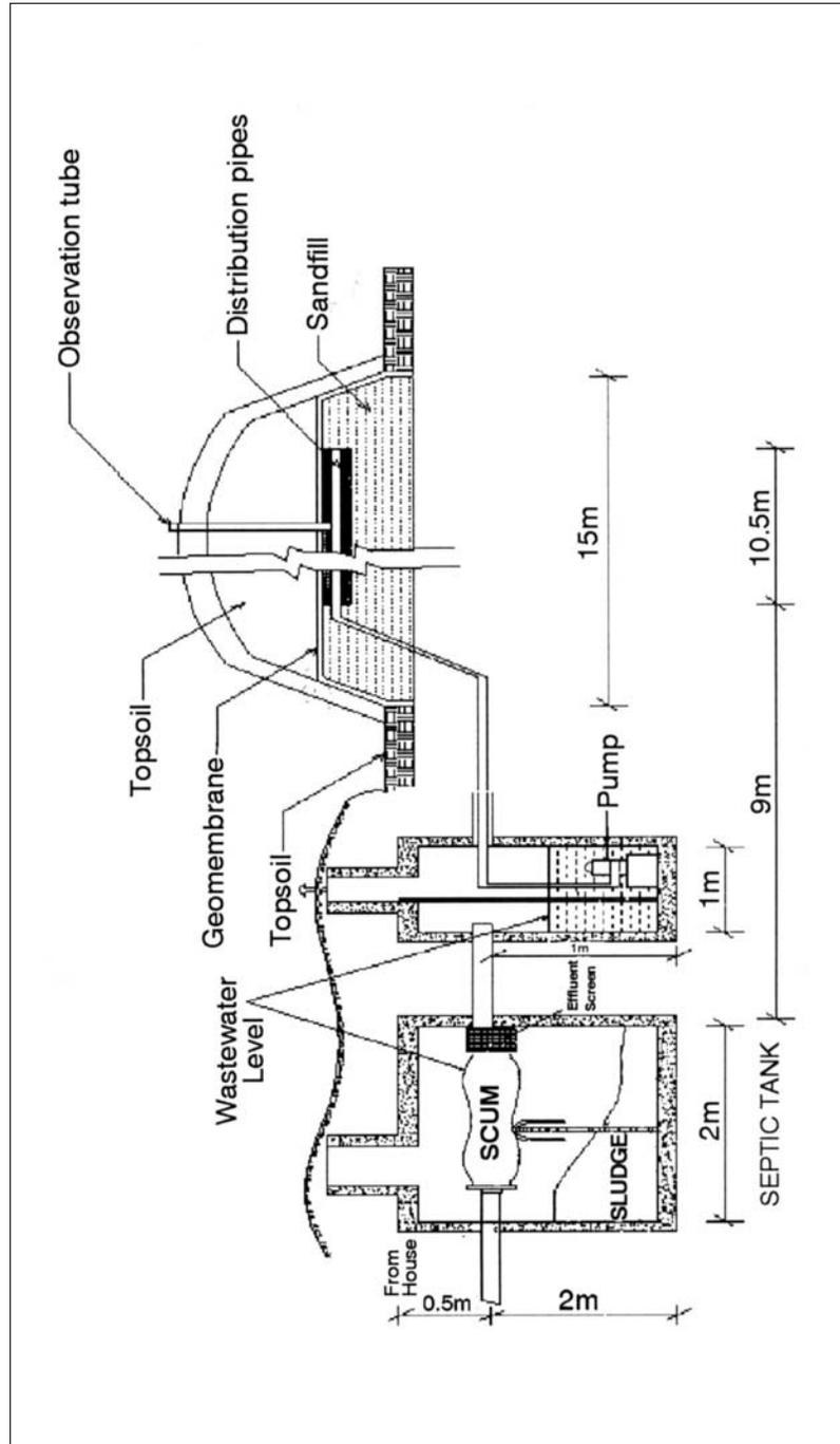
Figure 6. Section through on-site wastewater treatment system.
