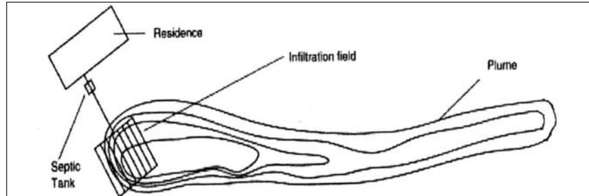
Figure 2. An example of effluent plume movement.
