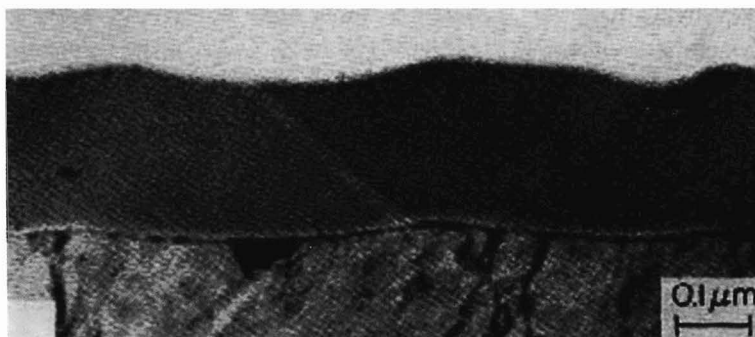
Fig. 1 SEM image of a cross section of an amorphous aluminium oxide layer (top) grown on aluminium (bottom) in 0.16 M ammonium tartrate at 20°C with a current density of 10 mA/cm 2 , voltage of 200 V. The oxide thickness is about 220 nm, equivalent to 1.1 nm/V [53]
