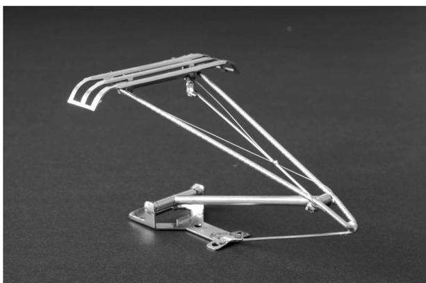
Figure 4: Close-up photograph of the used pantograph.
