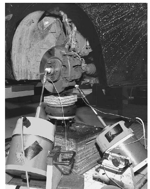
Figure 3. Multiple excitation of vehicle suspension with wheel and tyre removed
