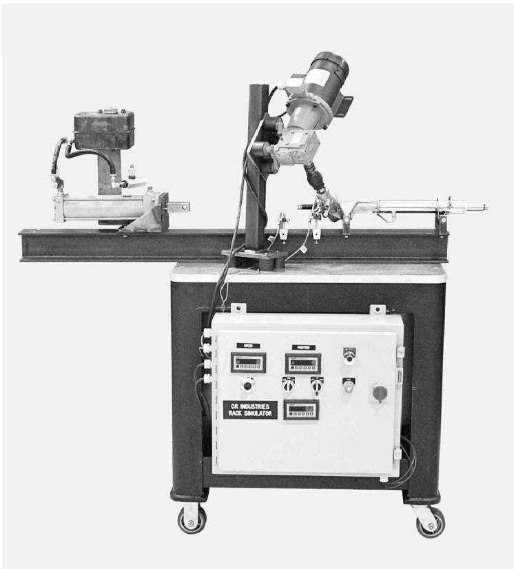
Figure 4. Steering gear simulator for laboratory testing
