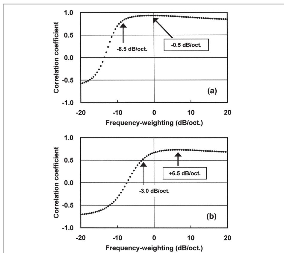
Figure 4. The trace of the correlation coefficient in estimating the 'best-fit' frequency-weighting for the  $VAL_{total}$  measured (a) at the chest and (b) at the abdomen (Experiment 1). The value shown in the rectangle is the slope of the 'best-fit' frequency-weighting estimated in the present study, while the other value is that estimated in the previous study (Ref. [20]).
