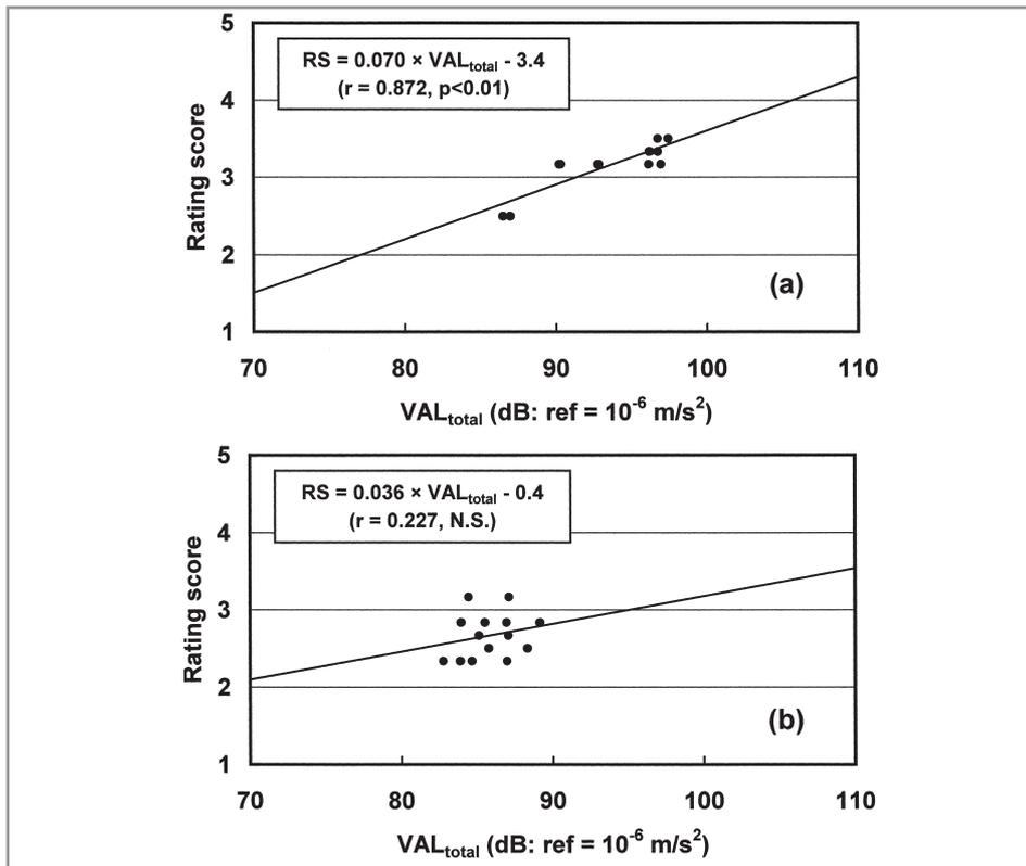
Figure 3. The correlation between the mean rating score (RS) of subjective unpleasantness and the mean VAL<sub>total</sub> of the body surface vibration measured (a) at the chest and (b) at the abdomen (Experiment 2).
