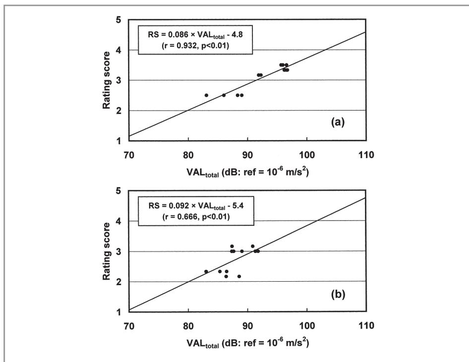
Figure 2. The correlation between the mean rating score (RS) of subjective unpleasantness and the mean  $VAL_{total}$  of the body surface vibration measured (a) at the chest and (b) at the abdomen (Experiment 1).
