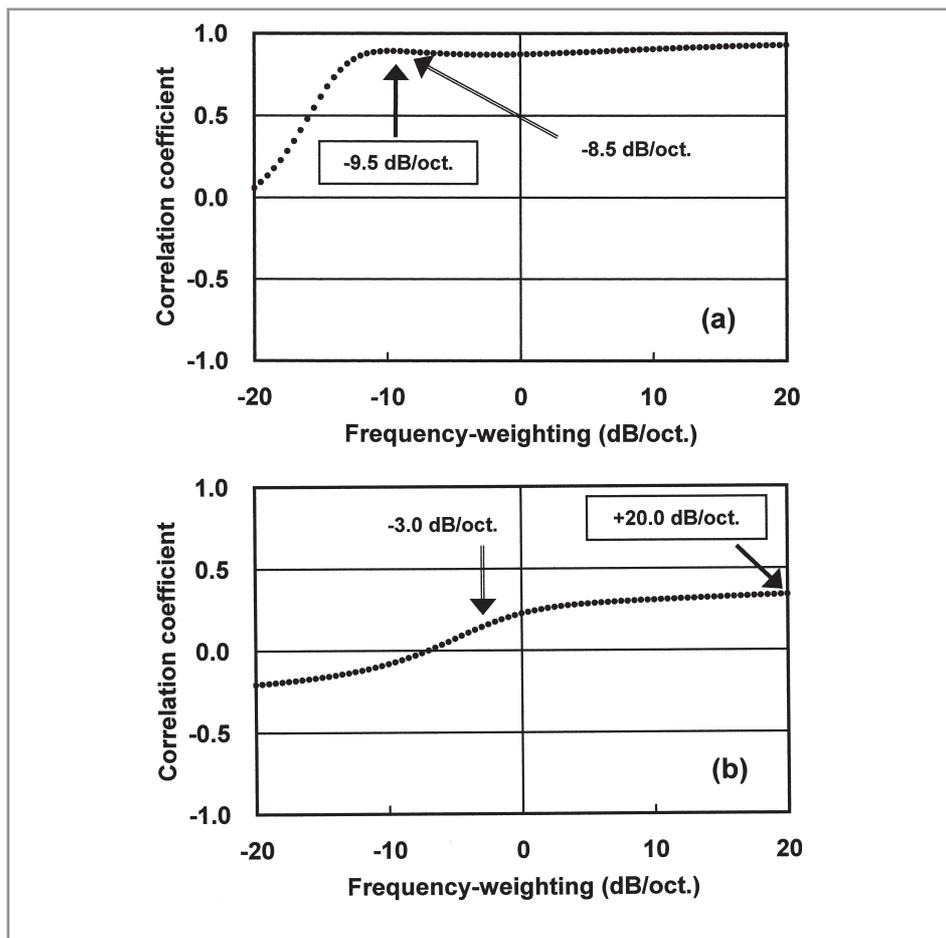
Figure 5. The trace of the correlation coefficient in estimating the ‘best-fit’ frequency-weighting for the  $VAL_{total}$  measured (a) at the chest and (b) at the abdomen (Experiment 2). For the two values shown in the figure, see the Fig. 4 caption.
