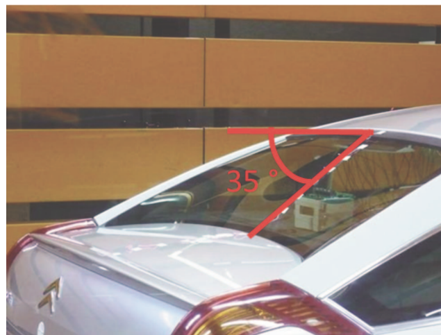
Figure 2. Rear window geometry details with mean slant angle in the symmetry plane
