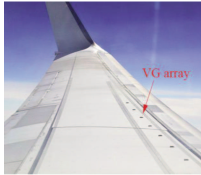
Figure 1. An array of vane-type VGs on the aircraft wing for shock buffeting control (photo taken on a B737-800 operated by Transavia flying from Barcelona to Amsterdam).
