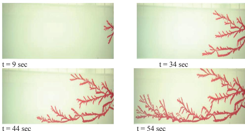
Figure 6. Displacement of 60% emulsion at injection rate 4.25 ml/min
