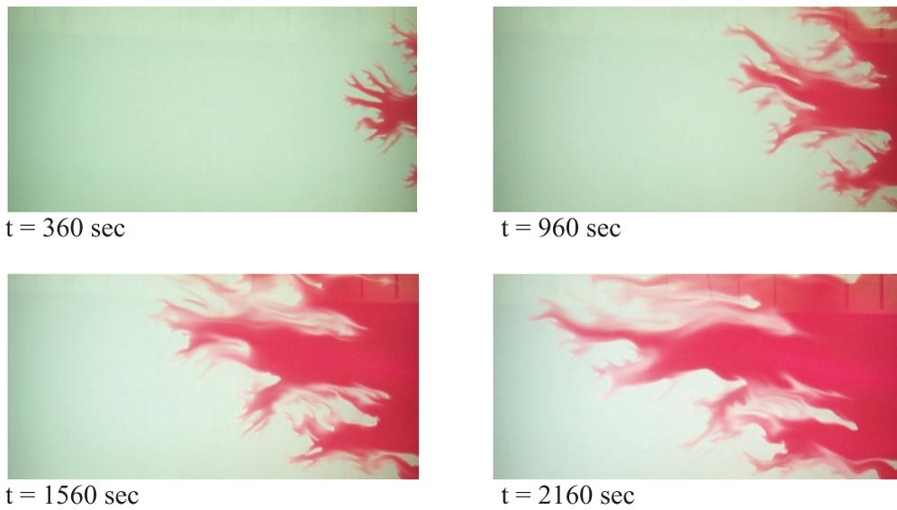
Figure 3. Displacement of 40% emulsion at injection rate 0.21 ml/min
