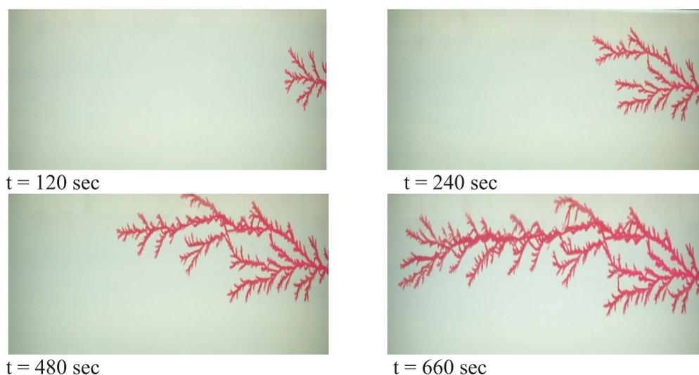
Figure 5. Displacement of 60% emulsion at injection rate 0.21 ml/min
