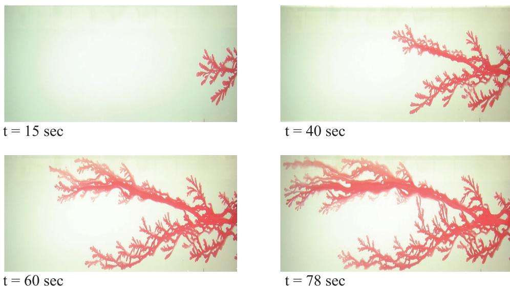
Figure 4. Displacement of 40% emulsion at injection rate 4.25 ml/min
