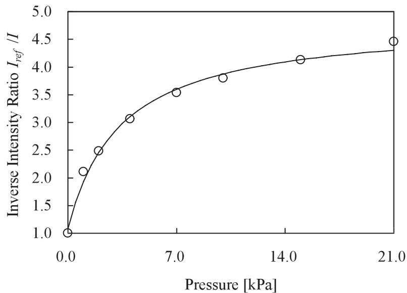
Figure 14. Stern-Volmer plots for PSMF composed of PtMP(○) and fitted curve
