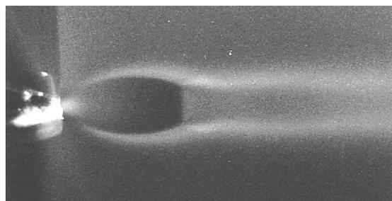
Figure 2. Supersonic free jet visualized by  $I_2$ -LIF
