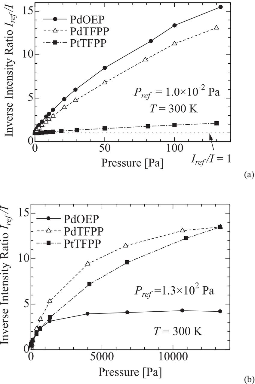
Figure 10. Stern-Volmer plots of PSPs, (a) Low pressure condition, (b) High pressure condition
