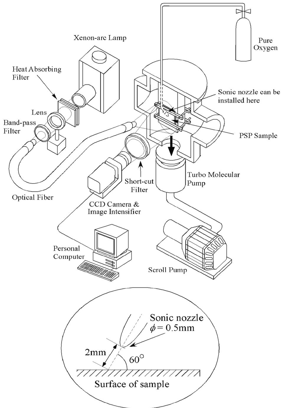
Arrangement of the nozzle and the PSP sample (when the nozzle is installed)
