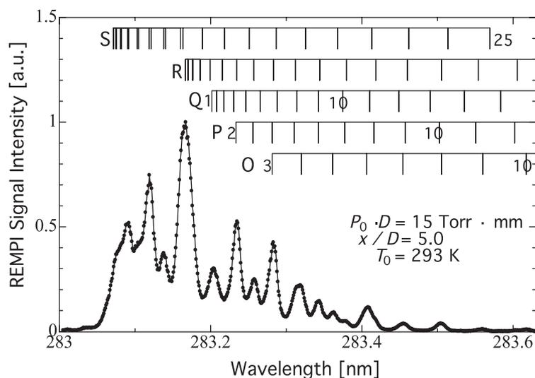
Figure 5. 2R+2  $N_2$ -REMPI spectrum for  $P_0 D = 15$  Torr mm and at  $x/D = 5$
