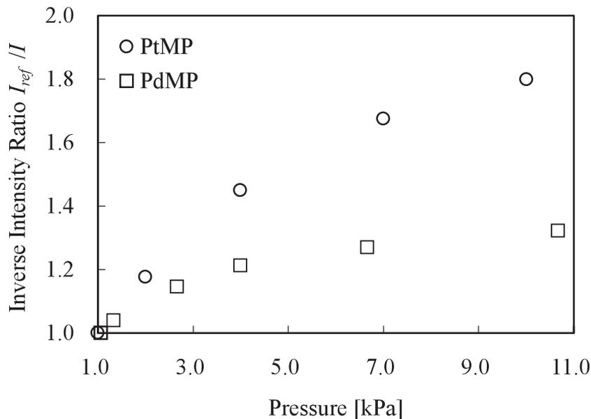
Figure 13. Stern-Volmer plot for the 2-layer PSMF composed of PtMP(○) and PdMP(□) below 11kPa, where  $I_{ref}$  is the luminescent intensity at  $P_{ref}$  ( $= 1.0\text{kPa}$ )
