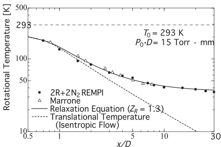
Figure 7. Rotational temperature distributions along the centerline of the jet ( $P_0 D=15$  Torr mm)
