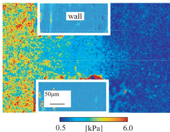
Figure 15. Pressure field of micro-channel obtained by PSMF composed of PtMP
