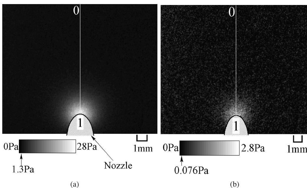
Figure 11. Pressure distribution measured by PdOEP, (a)  $P_0 = 1.3 \times 10^3$  Pa (10 Torr), (b)  $P_0 = 1.3 \times 10^2$  Pa (1 Torr)
