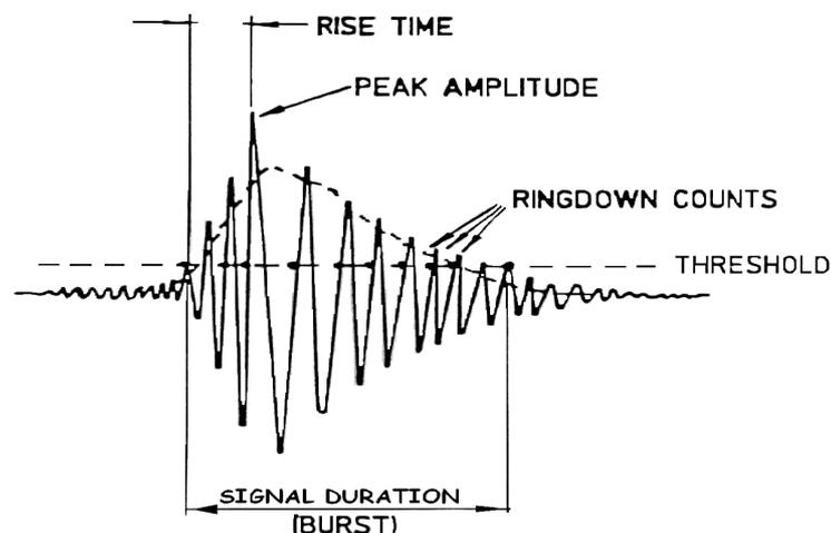
Figure 1. Acoustic Emission Parameters of a Typical Signal
