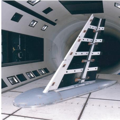
Figure 1. Trapezoidal Wing in 12ft test section, NASA Ames
