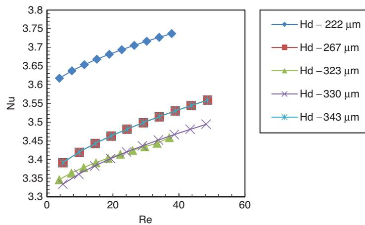
Figure 6. Nu number Vs Re number for  $L = 50$  mm
