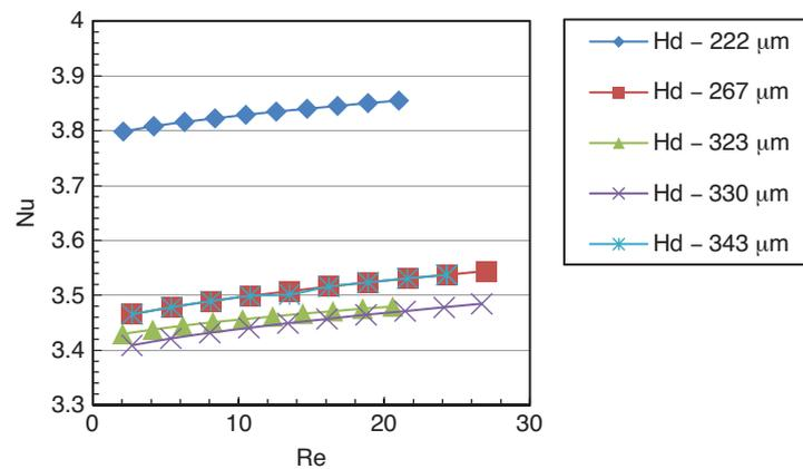
Figure 3. Nu number Vs Re number for L = 90 mm
