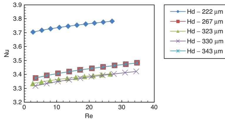
Figure 7. Nu number Vs Re number for L = 70 mm
