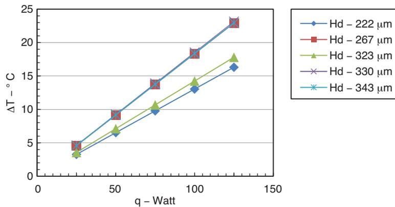
Figure 11. Temperature diff. Vs Heat input for flow rate of 0.167 kg/sec, L = 50 mm
