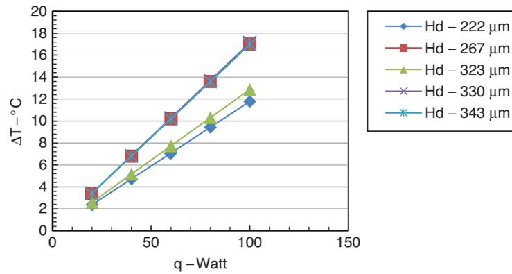
Figure 12. Temperature diff. Vs Heat input for flow rate of 0.0167 kg/sec, L = 50 mm
