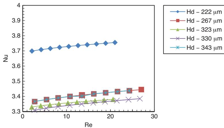
Figure 8. Nu number Vs Re number for L = 90 mm
