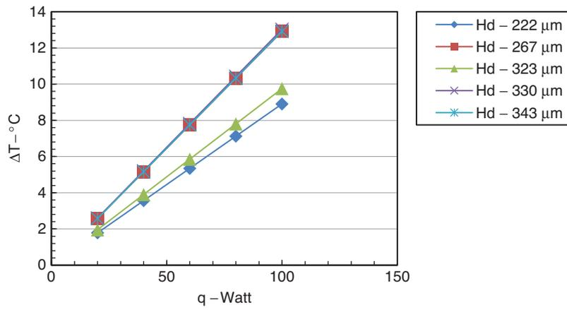
Figure 16. Temperature diff. Vs Heat input for flow rate of 0.067 kg/sec, L = 90 mm
