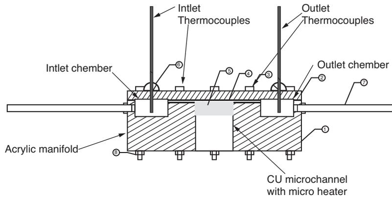
Figure 5. Microchannel test section manifold
