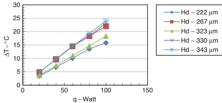
Figure 9. Temperature diff. Vs Heat input for flow rate of 0.0167 kg/sec, L = 50 mm
