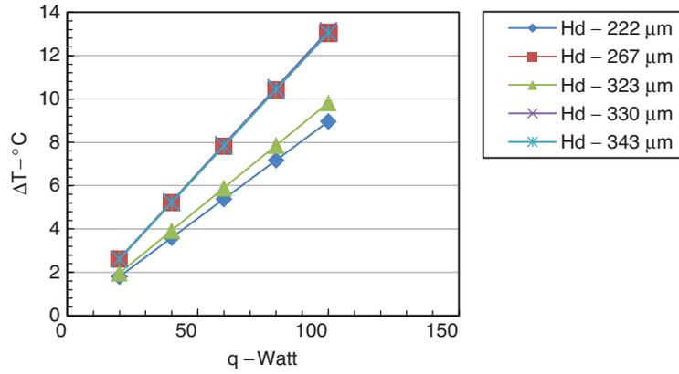
Figure 15. Temperature diff. Vs Heat input for flow rate of 0.0167 kg/sec, L = 90 mm
