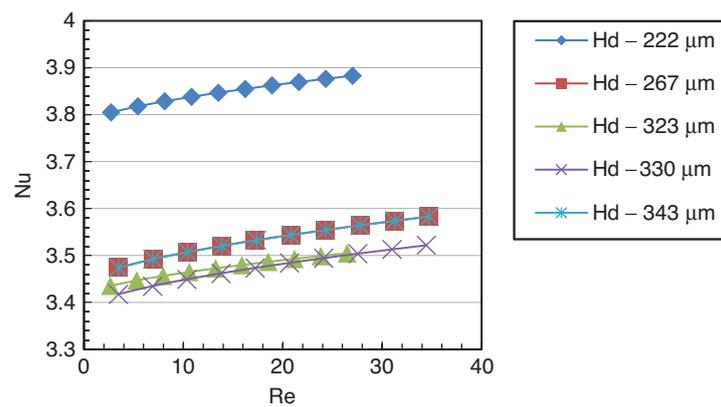
Figure 2. Nu number Vs Re number for L = 70 mm
