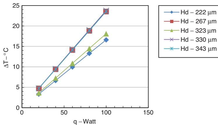
Figure 10. Temperature diff. Vs Heat input for flow rate of 0.067 kg/sec, L = 50 mm
