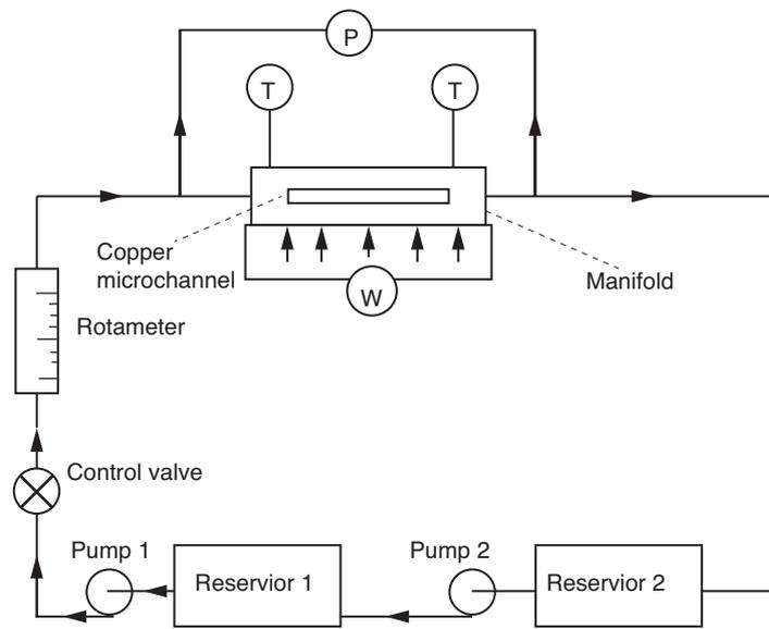
Figure 4. Flow loop of Experimental Test set up
