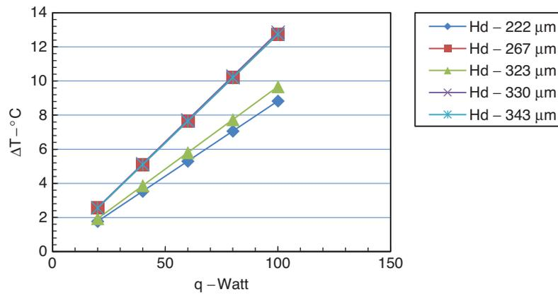
Figure 17. Temperature diff. Vs Heat input for flow rate of 0.167 kg/sec, L = 90 mm
