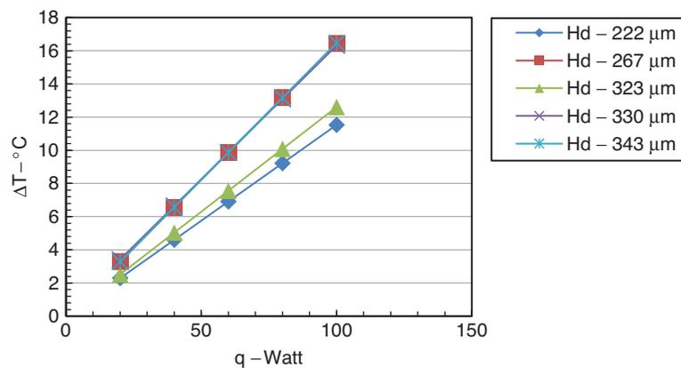
Figure 14. Temperature diff. Vs Heat input for flow rate of 0.167 kg/sec, L = 70 mm
