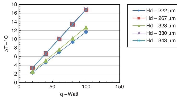
Figure 13. Temperature diff. Vs Heat input for flow rate of 0.067 kg/sec, L = 70 mm
