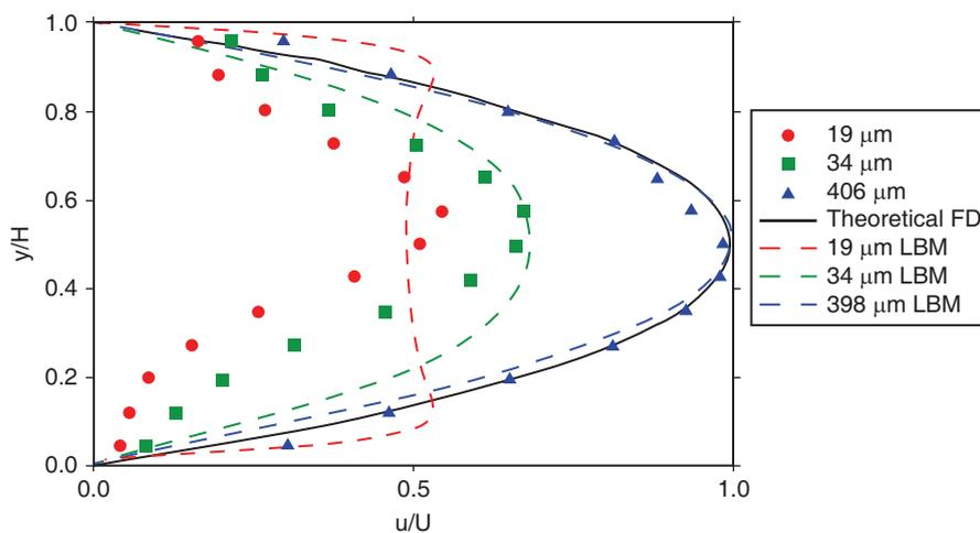
Figure 2. Comparison of developing velocity profiles with Ahmad and Hassan [6] for  $D_h = 100$  mm and  $Re = 50$
