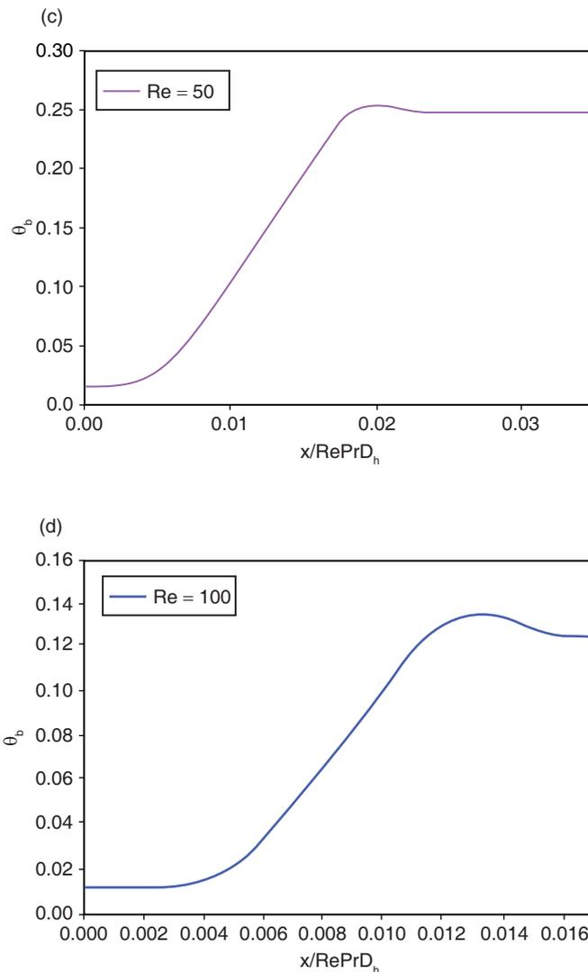
Figure 5. Development of non-dimensional bulk mean temperature with non-dimensional axial distance for  $D_h = 100$ mm (a)  $Re = 5$ , (b)  $Re = 10$ , (c)  $Re = 50$  and (d)  $Re = 100$
