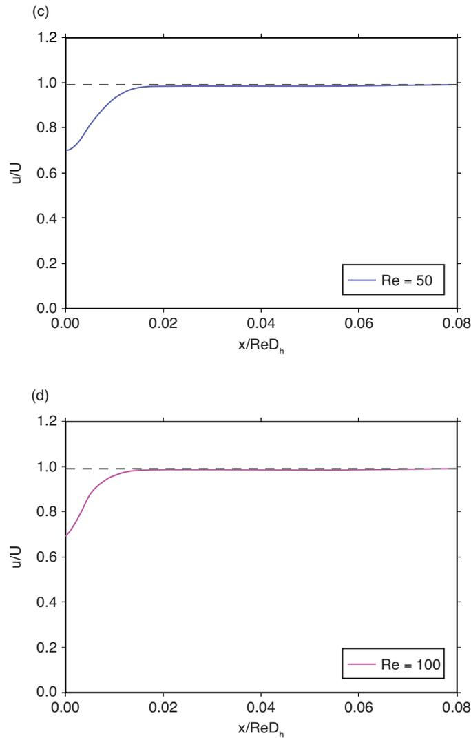
Figure 3. Development of centerline velocity for  $D_h = 100$  mm (a)  $Re = 5$ , (b)  $Re = 10$ , (c)  $Re = 50$  and (d)  $Re = 100$
