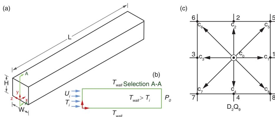
Figure 1. (a) Schematic of microchannel geometry (b) Computational domain for present study (c)  $D_2Q_9$  Lattice arrangement
