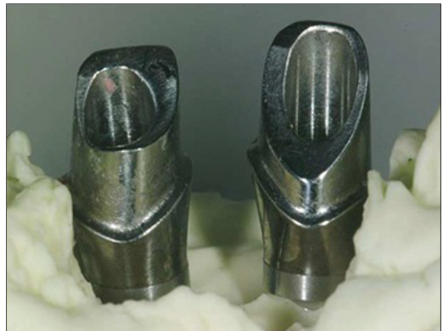
Figure 15: Close examination of the abutments shows a smooth marginal chambers and excellent abutment/analog interfaces
