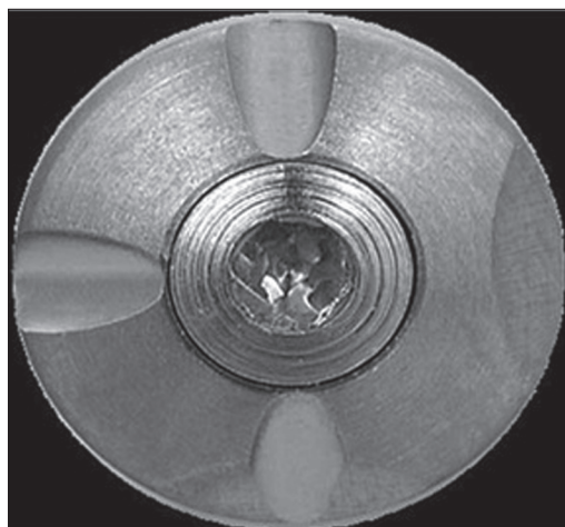
Figure 5: Unique encoded healing abutments are read by an optical scanner to determine the implant size, hex position, implant location, and soft tissue levels
