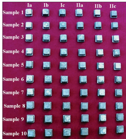
Figure 5: Samples fabricated after two different casting techniques, that is, ringless and closed ring casting techniques using three different base metal alloys (Mealloy, Wiron 99 and Bellabond plus)
