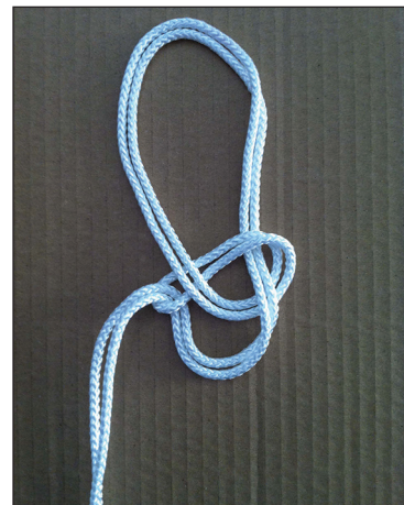
Figure 3: The Nice knot is a double-stranded knot, which increases bulk. It was tested with 0, 1, 2, and 3 half-hitches. Shown without half-hitches
