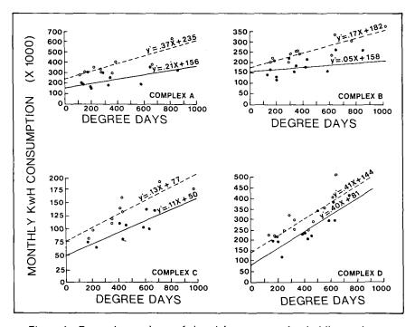
Figure 1. Regression analyses of electricity consumption in kilowatt-hours (KwH) as a function of degree days (absolute values of heat days plus cool days) before and after conversion from master metering to individual metering for the four apartment complexes examined in this study (Note: closed circles signify before conversion; open circles signify after conversion).
