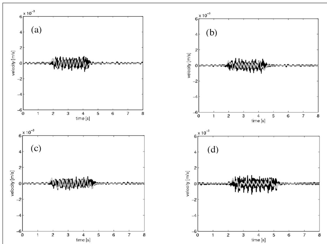
Figure 3. Vertical velocity at a point 8 m from the track: (a)  $v=315$  km/h (b)  $v=300$  km/h (c)  $v=271$  km/h (d)  $v=256$  km/h. Experimental (black line) vs. Numerical (grey line)
