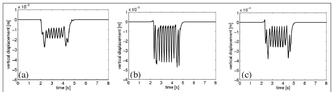
Figure 8. Vertical displacement at three points located 11.45 m from the track axis due to the passage of an Alstom HST with  $v = 300$  km/h: (a)Point A1 (b)Point A2 (c)Point A3.
