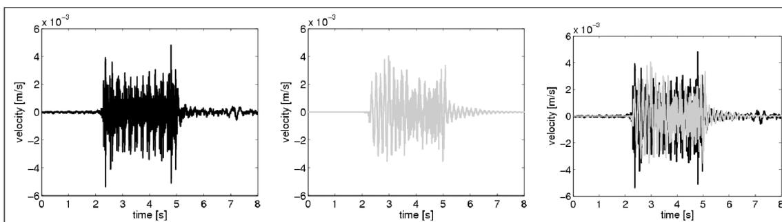
Figure 6. Time history of the vertical velocity in the support structure at the passing of an AVE-Alstom train travelling at a speed,  $v=298$  km/h on Track 1. Experimental Result (black line) vs. Numerical Result (grey line)
