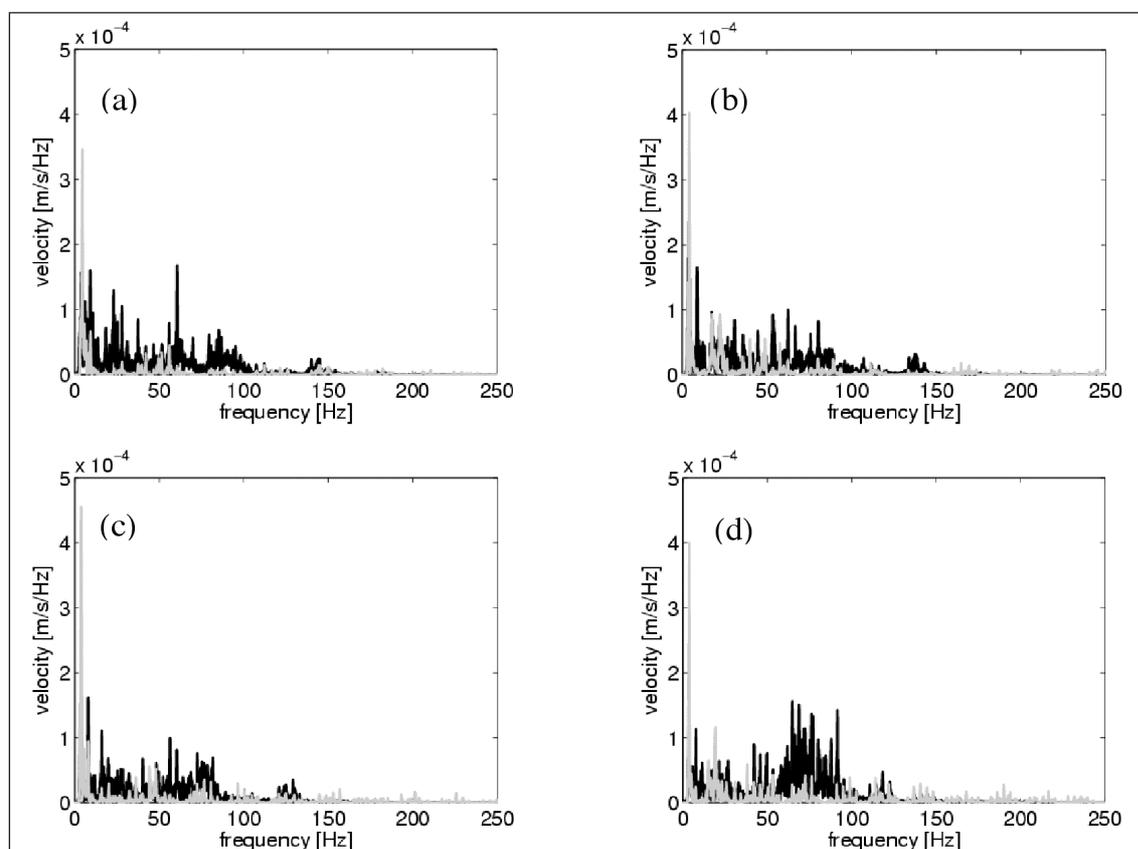
Figure 4. Frequency content of the vertical velocity at a point 8 m from the track: (a)  $v=315$  km/h (b)  $v=300$  km/h (c)  $v=271$  km/h (d)  $v=256$  km/h. Experimental (black line) vs. Numerical (grey line)
