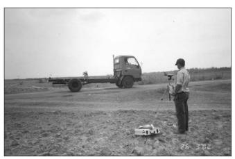
Figure 4. Passby noise measurements of a truck at a test track
