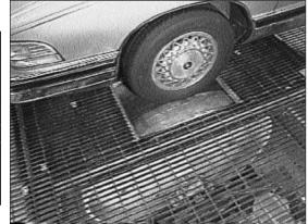
10. View of a chassis roll dynamometer [16]
