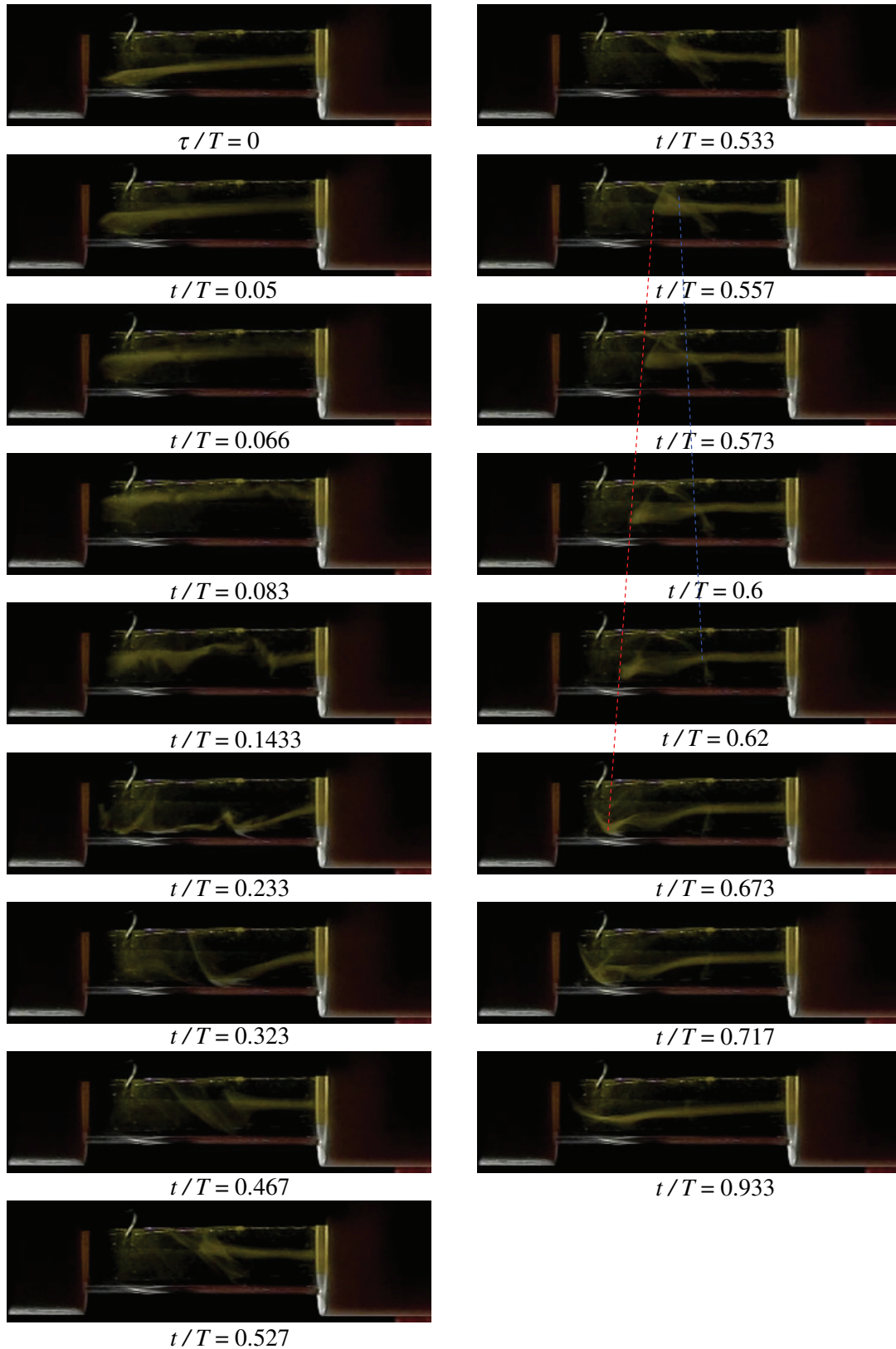
Figure 13. Smoke filament flow visualization at f^+ = 0.34 , filmed at 1200fps photography.
