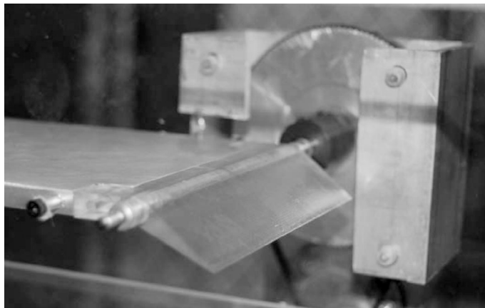
Figure 4. The flat plate flap with a stepper motor control.
