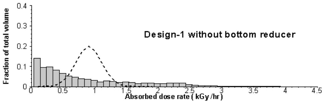
(d) Volumetric absorbed dose rate distribution for irradiator without bottom reducer
