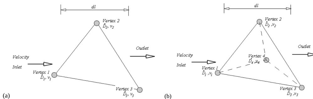
Figure 6. An illustration of (a) triangular (b) tetragonal element used in 2D and 3D analysis.
