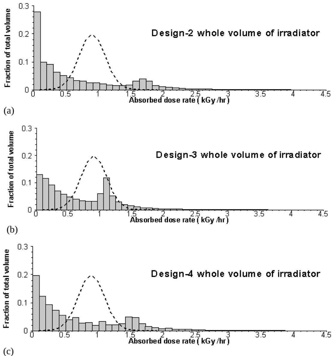
Figure 10. Volume averaged dose rate distribution for (a) design-2, (b) design-3 and (c) design-4.
