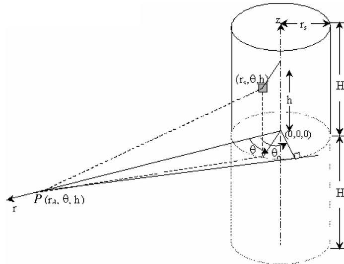
Figure 3. The calculation of dose rate for a cylindrical source of finite length.
