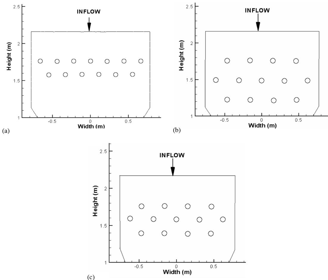
Figure 8. The cross-section view near the source assembly for (a) design-2, (b) design-3 and (c) design-4.
