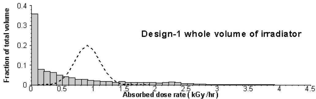
(c) Volumetric absorbed dose rate distribution for whole volume of irradiator
