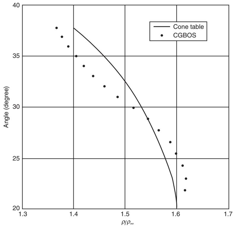
Figure 15. Comparison of normalized density behind the shock.
