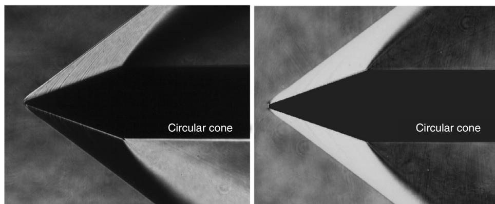
Figure 9. Conventional schlieren images, taken with horizontal knife-edge (left) and taken with vertical knife-edge (right).
