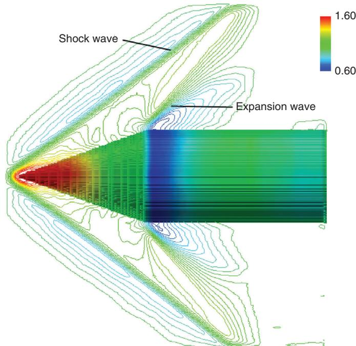
Figure 13. Reconstructed density distribution ( $\rho/\rho_0$ ): contour on a central plane and pseudo-color near the surface of circular cone.
