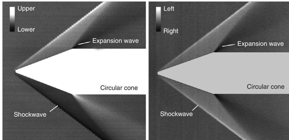
Figure 8. Gray-scale images of calculated displacement, vertical displacement of background obtained from horizontal green stripe (left) and horizontal displacement obtained from vertical red stripe shown in Fig. 7.
