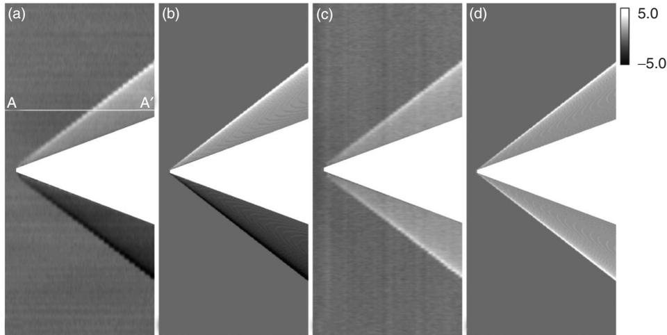
Figure 10. Comparison between CGBOS displacement image and pseudo-CGBOS image obtained with density distribution from cone table [18]; (a) Vertical displacement obtained from CGBOS (shown in Fig. 8), (b) Pseudo image of vertical displacement calculated from cone table, (c) Horizontal displacement from CGBOS (shown in Fig. 8), (d) Pseudo image of horizontal displacement calculated from cone table [18].
