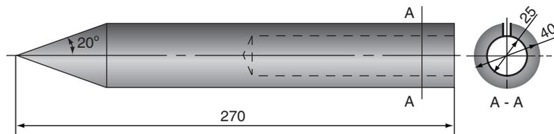
Figure 3. Test model (circular cone).
