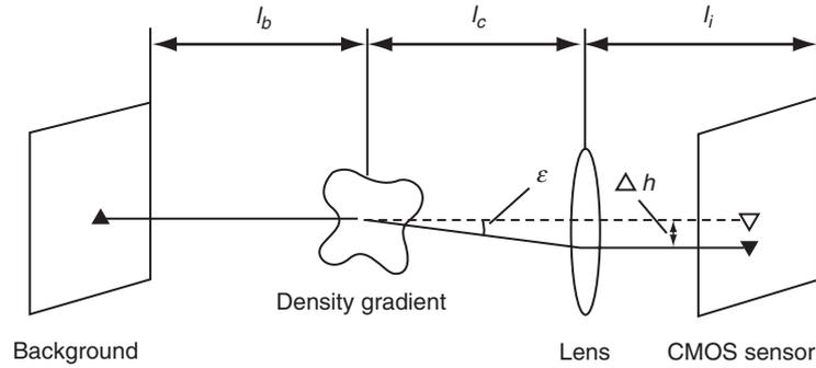
Figure 1. Optical setup of BOS measurement.
