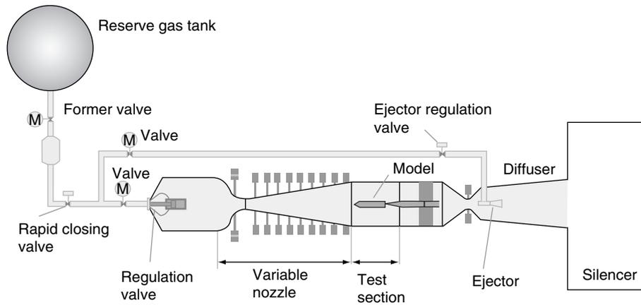
Figure 2. Supersonic wind tunnel at JAXA/ISAS.
