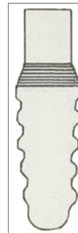
Figure 6: Implant with a reverse conical neck
