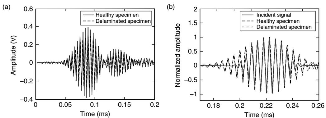
Figure 15. T-pull specimen (a) Forward propagating  $S_0$  mode picked up by sensor (b) Time reversed  $S_0$  mode picked up by sensor.
