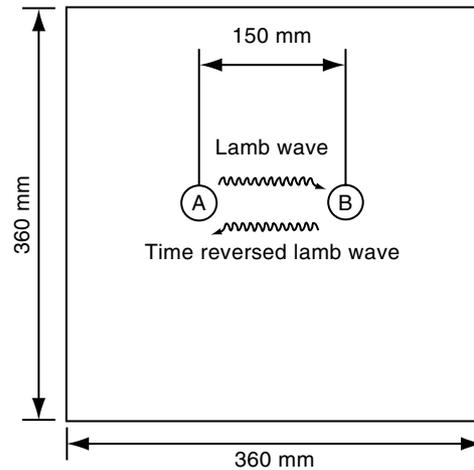
Figure 4. Schematic diagram of the composite plate with PZT sensors.
