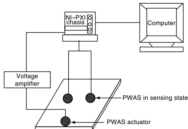
Figure 3. Schematic diagram of the experimental setup.
