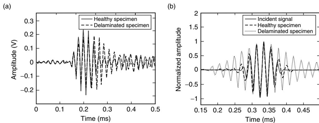
Figure 14. T-pull specimen (a) Forward propagating  $A_0$  mode picked up by sensor (b) Time reversed  $A_0$  mode picked up by sensor.
