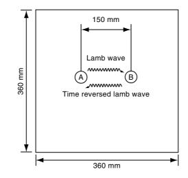
Figure 4. Schematic diagram of the composite plate with PZT sensors.
