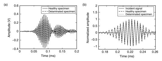
Figure 15. T-pull specimen (a) Forward propagating  $S_0$  mode picked up by sensor (b) Time reversed  $S_0$  mode picked up by sensor.
