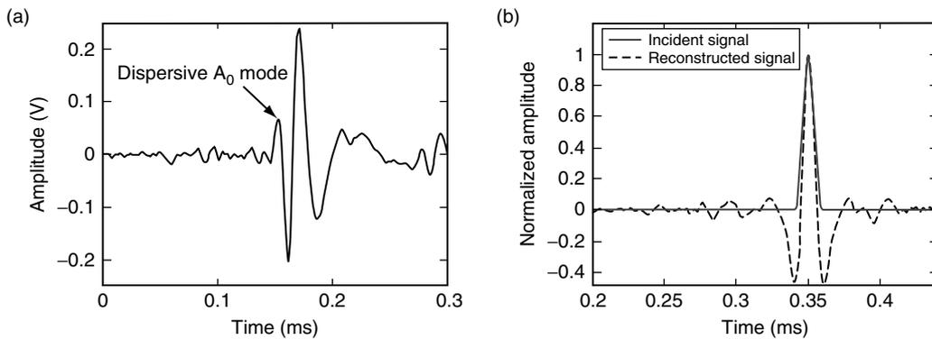
Figure 5. Unidirectional glass-epoxy composite (a) Signal picked up by sensor B under Gaussian pulse (b) Reconstructed signal at sensor A.
