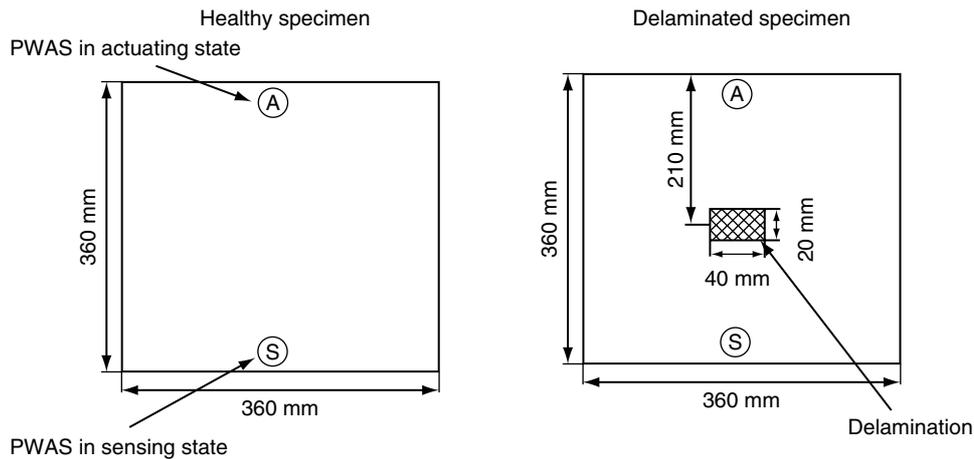
Figure 11. Schematic diagram of the healthy and delaminated unidirectional glass-epoxy composite plate with PWAS sensors.
