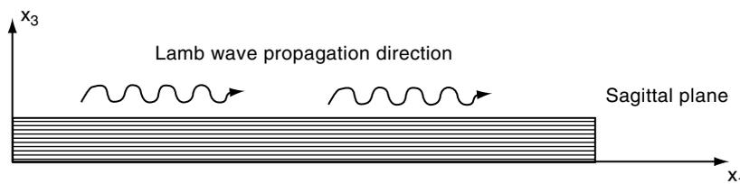
Figure 1. Schematic diagram of Lamb wave propagation in Composite laminate.
