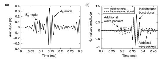
Figure 10. Cross ply glass-epoxy composite plate under narrow band excitation: (a) Forward propagating Lamb wave picked up by the sensor (b) Reconstructed time reversed Lamb wave picked up by sensor.
