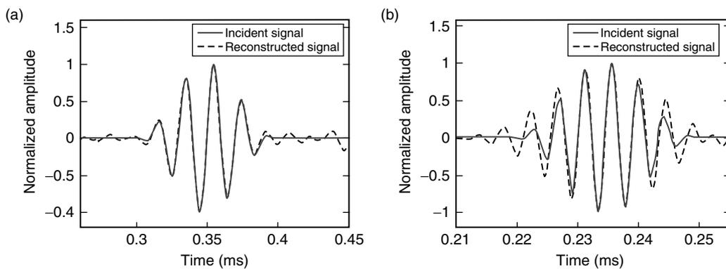
Figure 6. Unidirectional glass-epoxy composite: Time reversed signal picked up by sensor A (a)  $A_0$  mode (b)  $S_0$  mode.
