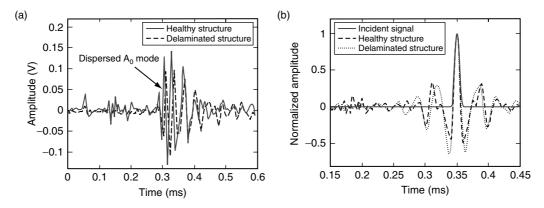
Figure 12. Unidirectional glass-epoxy composite with delamination under Gaussian pulse excitation: (a) Forward propagating Lamb wave picked up by the sensor (b) Reconstructed time reversed Lamb wave picked up by sensor.
