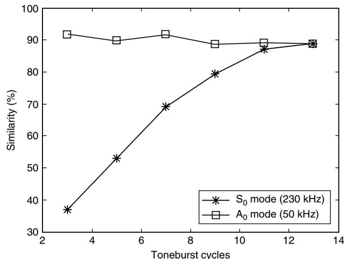
Figure 7. Unidirectional glass/epoxy composite: Similarity coefficient versus tone burst cycles.
