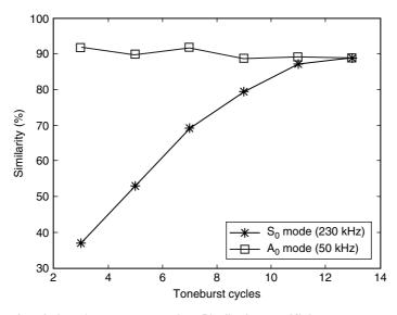
Figure 7. Unidirectional glass/epoxy composite: Similarity coefficient versus tone burst cycles.
