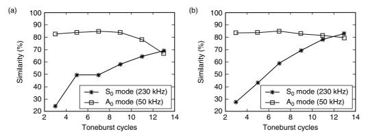
Figure 8. Similarity coefficient plot for glass-epoxy composite (a) Crossply (b) Quasi-isotropic.
