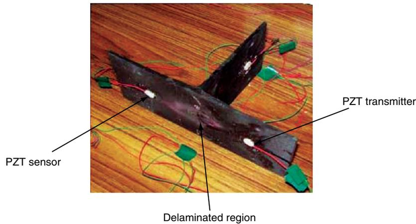
Figure 13. T-pull composite specimen with surface bonded PZT sensors.
