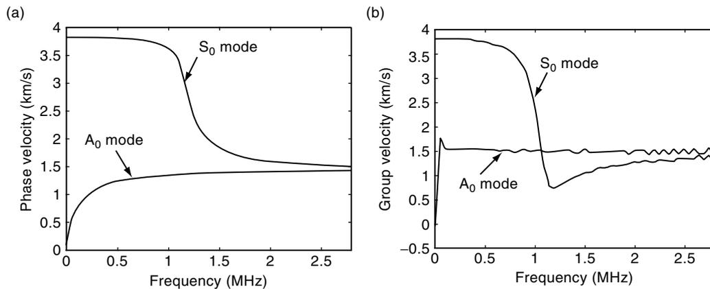
Figure 2. Dispersion curves for Uni-directional Glass/epoxy composite beam (a) Phase velocity vs. Frequency (b) Group velocity vs. Frequency.
