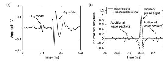
Figure 9. Cross ply glass-epoxy composite plate under Gaussian pulse excitation: (a) Forward propagating Lamb wave picked up by the sensor (b) Reconstructed time reversed Lamb wave picked up by sensor.
