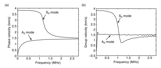
Figure 2. Dispersion curves for Uni-directional Glass/epoxy composite beam (a) Phase velocity vs. Frequency (b) Group velocity vs. Frequency.
