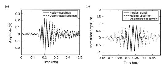
Figure 14. T-pull specimen (a) Forward propagating  $A_0$  mode picked up by sensor (b) Time reversed  $A_0$  mode picked up by sensor.
