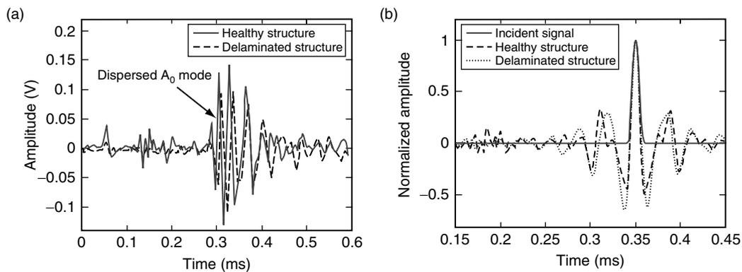
Figure 12. Unidirectional glass-epoxy composite with delamination under Gaussian pulse excitation: (a) Forward propagating Lamb wave picked up by the sensor (b) Reconstructed time reversed Lamb wave picked up by sensor.
